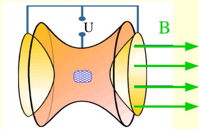
axial confinement by an electrostatic field
