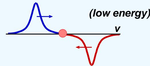
**synchronous velocity**  $v_s = C \cdot f_b / h$
