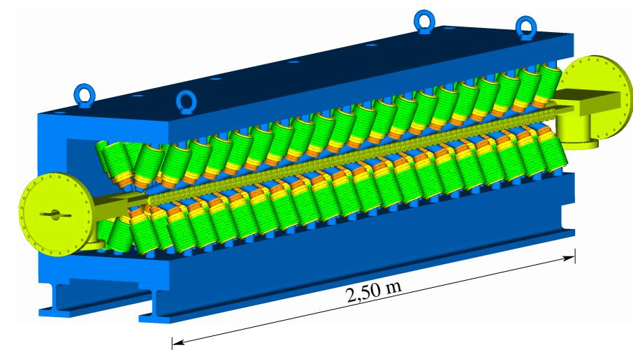
→ simultaneous cooling of two velocity projections inside and outside the helical wiggler
