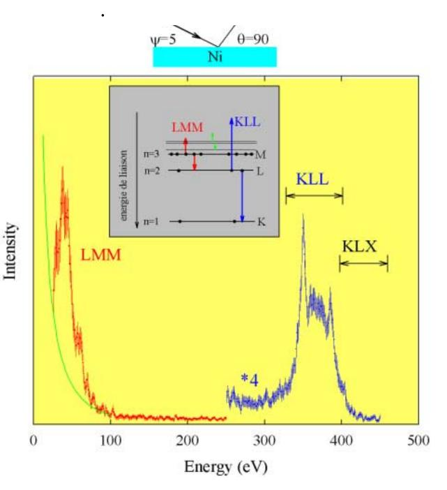
Typical Auger-electron Spectrum resulting from N<sup>6+</sup> collisions on Ni
