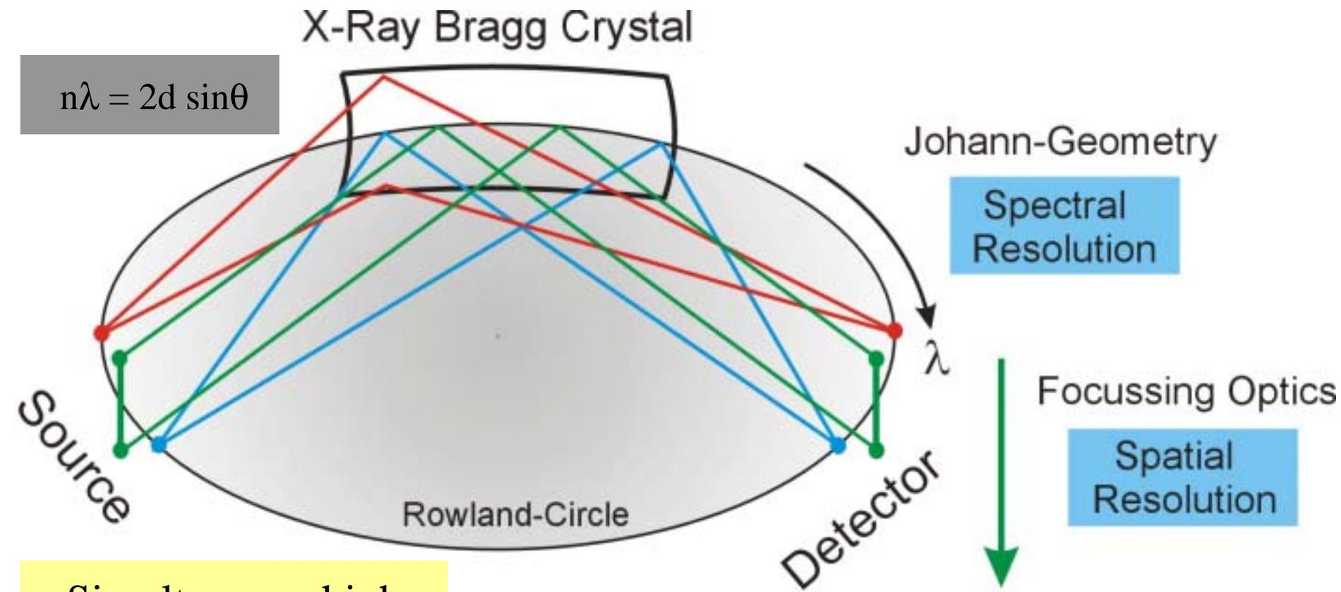
Simultaneous high spectral and spatial resolution while maintaining high luminosity (*no slit !*)
