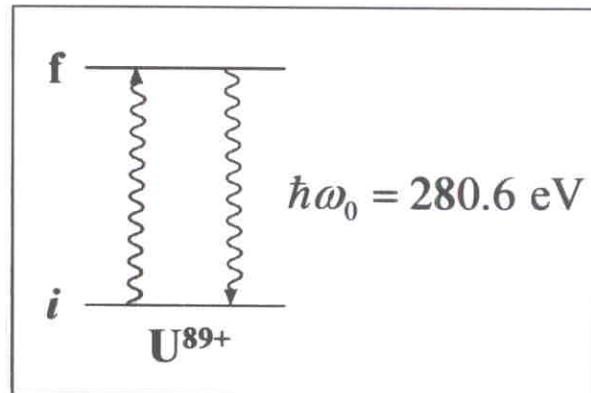
**Laser**       $\hbar\omega_L = \sqrt{\frac{1-\beta}{1+\beta}} \cdot \hbar\omega_0 \underset{\gamma \gg 1}{\approx} \frac{\hbar\omega_0}{2\gamma} = 5.87 \text{ eV}$
