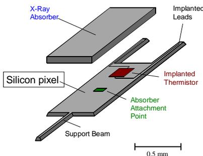
Fig. 1: Schematic view of one pixel of the calorimetric low-temperature detector.
