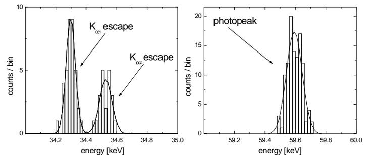
Fig. 3: Energy spectrum measured with a calorimetric detector at an operating temperature of 60 mK with a  $0.3 \text{ mm}^2 \times 66 \mu\text{m}$  Sn absorber for 59.6 keV photons. An energy resolution of  $\Delta E_{\text{FWHM}} = 121$  eV for the photopeak (right side) and of  $\Delta E_{\text{FWHM}} = 72$  eV for the  $K_{\alpha}$  escape lines (left side) is obtained.
