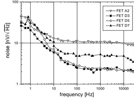
Fig. 2: Noise spectra measured at  $T = 125$  K for different samples of two modifications (A, D) of FET's of the type INTERFET NJ14AL.
